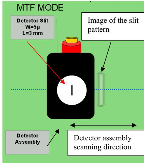
Figure 3: Diagrammatic view of the focal plane of the lens to be tested.
