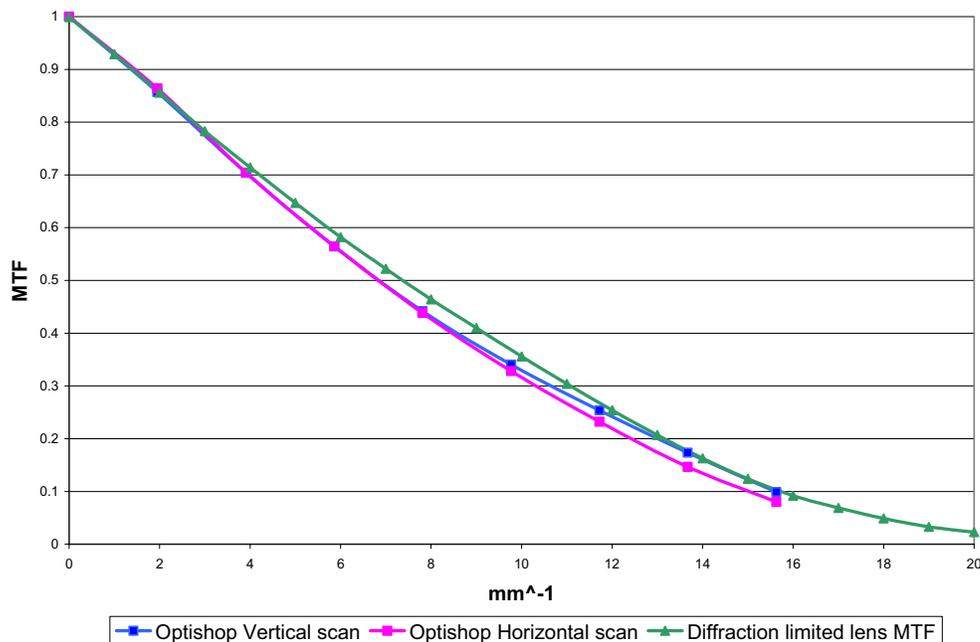
Figure 7: On-axis MTF measurement with the OPTISHOP system of an 8-12 $\mu$  lens (Ge singlet close to diffraction limit) versus theoretical diffraction-limited MTF curve. The lens is an EFL 252 mm., entrance pupil 48 mm. Deviations are  $\sim\pm 3\%$ .
