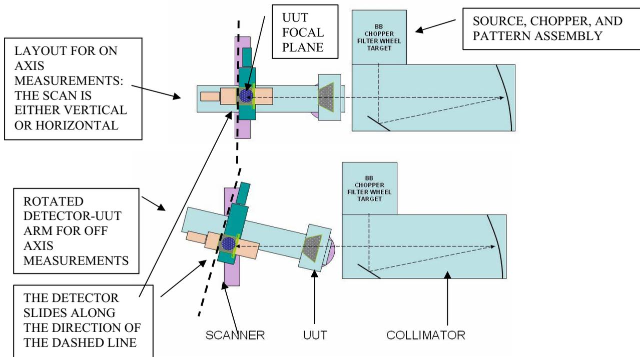
Figure 1: Optical layout diagram of the assembled OPTISHOP system. The lower diagram shows the system when the detector-UUT arm is rotated to perform off-axis measurements. The rotation is around a vertical axis going through the lens to be tested.
