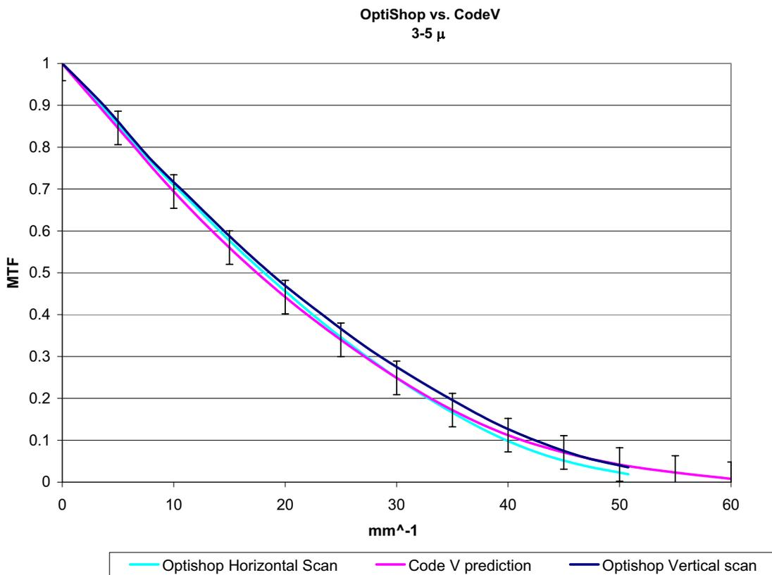
Figure 6: On-axis MTF measurement with the OPTISHOP system of a 3-5 $\mu$  lens (Si/Ge doublet not diffraction limited) versus CODE V prediction. The lens is an EFL 250 mm., entrance pupil 48 mm. diameter. Deviations are  $\sim\pm 4\%$ .
