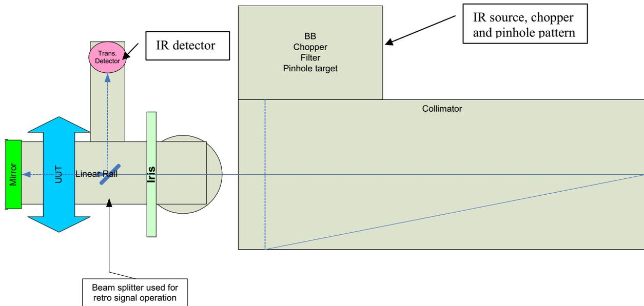
Figure 4: OPTISHOP optical layout for transmittance measurements. The collimated radiation from the source goes through an iris to match the illumination cross section with the lens diameter, then through a beamsplitter, through the UUT, it is reflected by a high reflectance mirror, back to the UUT and it is finally reflected by the beamsplitter to the IR detector. The reference measurement is done without the UUT in the path.
