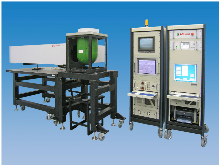
Figure 1: An example of electro-optical system mounted in a pod (green container) being tested by a CTE based test system. On the right are the control panels and computer.
