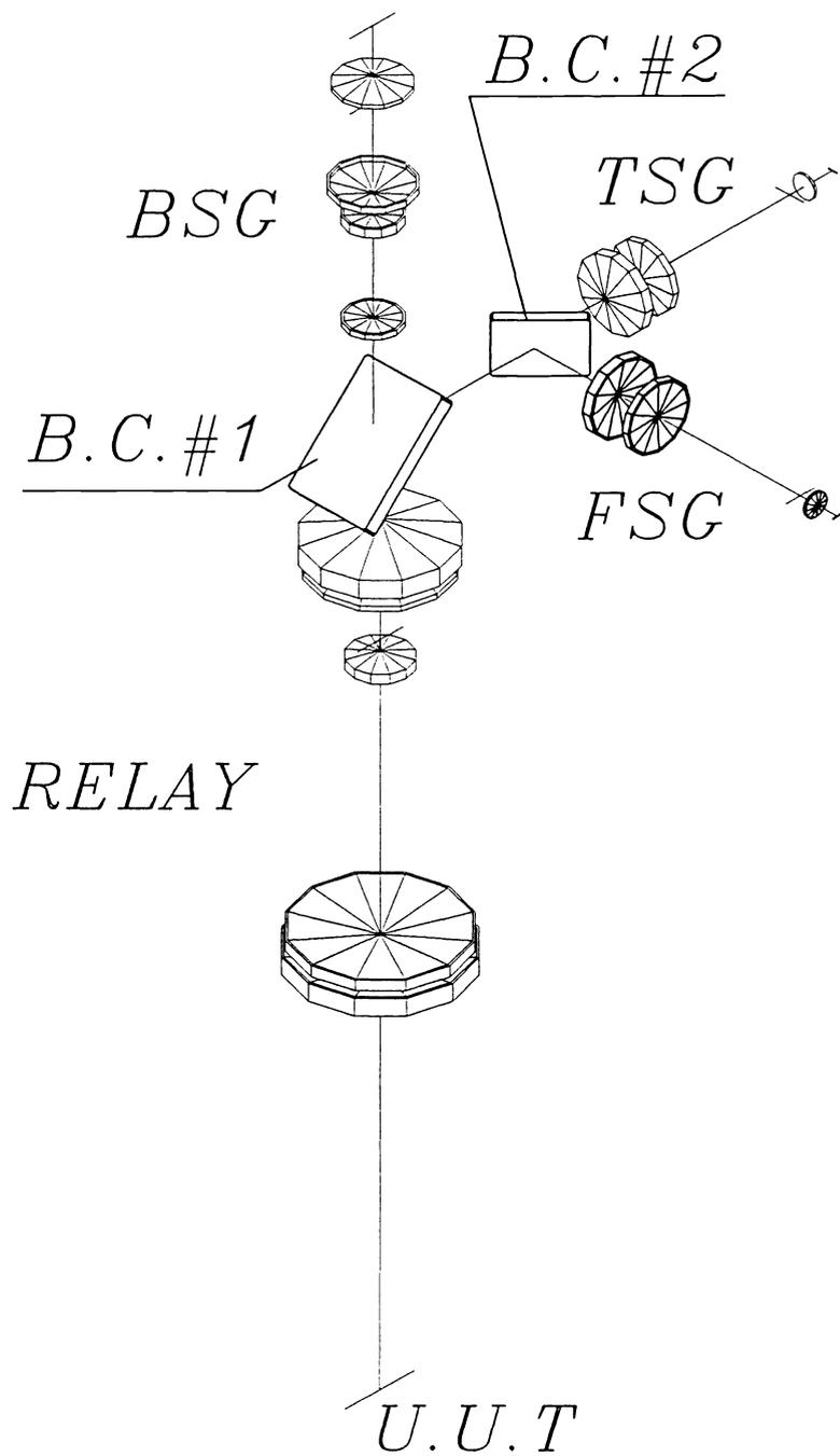
Figure 3: IRSG optical layout
