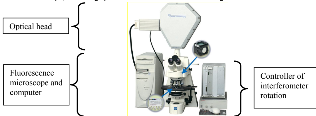
Figure 1: The SD 200 spectral imager, combined with a fluorescence microscope, being used for very advanced analysis and classification of genetic abnormalities, is not suitable for pushbroom operation.
