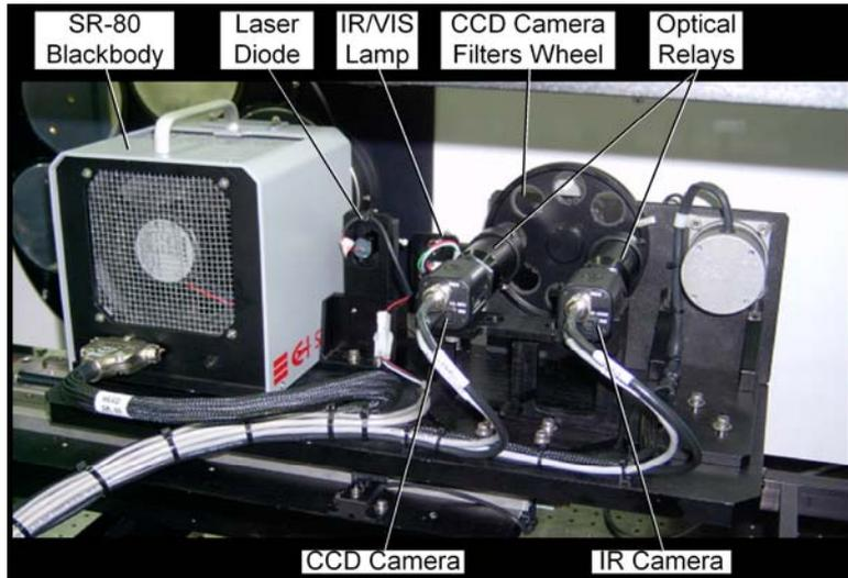
Figure 3: Typical EIRT collection of sources/sensors on the collimator focal plane.
