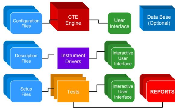
Figure 5: Block diagram of the EIRT software.
