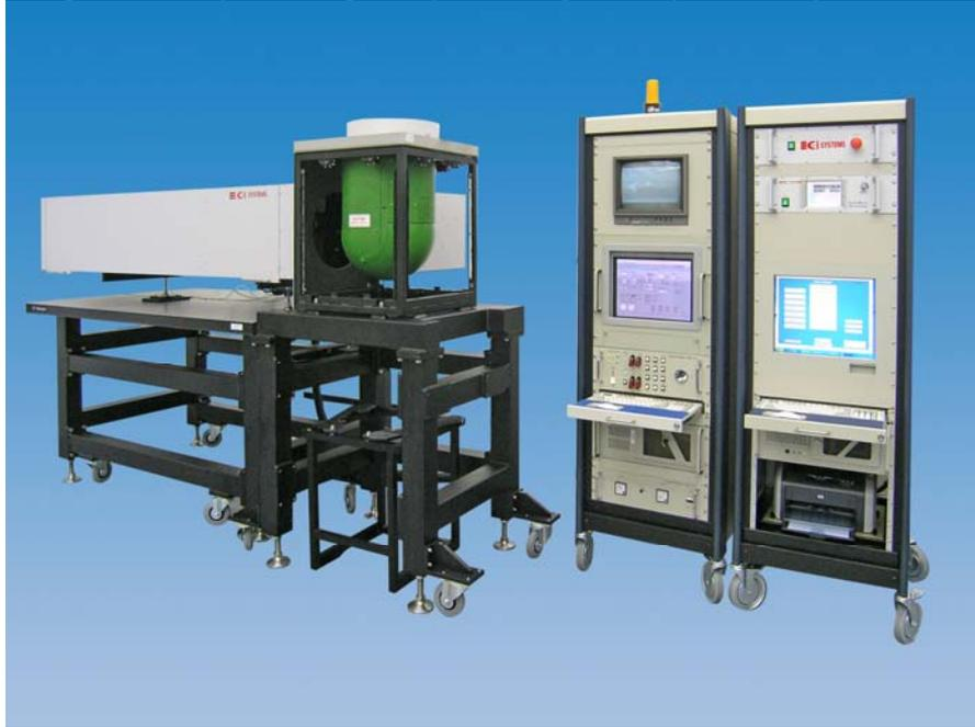
Figure 1: An example of electro-optical system mounted in a pod (green container) being tested by an EIRT test system. On the right are the control panels and computer.
