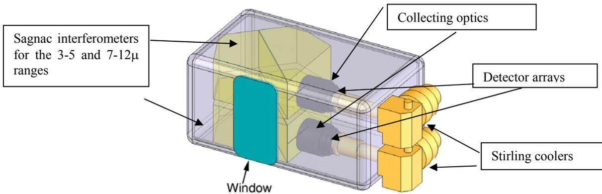
Figure 5: Conceptual view of the dual band IR spectral imager according to the present design. The small optics size and the fact that the collecting optics is made of only two units between the interferometers and the detector arrays, make the instrument especially compact and low cost.
