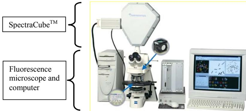
Figure 1: The SpectraCube™ spectral imager, combined with a fluorescence microscope, being used for very advanced analysis and classification of genetic abnormalities in cancer genetics studies.
