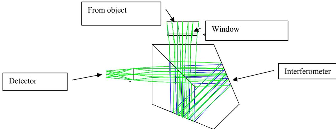
Figure 6: Monolithic interferometer design, avoiding any optical misalignment of the beamsplitter and interferometer mirrors, due to vibrations of any type.
