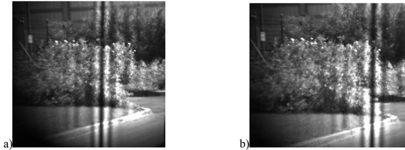
Figure 3: a) FOV frame at the central interferometer position (the central bright fringe is the "zero OPD" fringe); b) the same FOV scene, corresponding to an interferometer off-center angular position: since the interferometer is rotated, the central fringe is not on the central pixel column.
