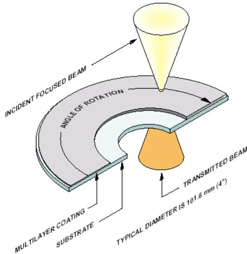
Figure 3: A typical CVF 1/2 disc segment, showing its active area and the cone of angle of the measured radiation (from OCLI's technical material).
