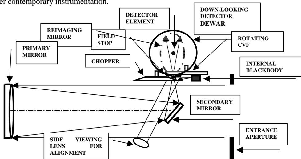
Figure 2: Optical layout of both the early SR 1000 model, and the later 5000 IR spectroradiometers.
