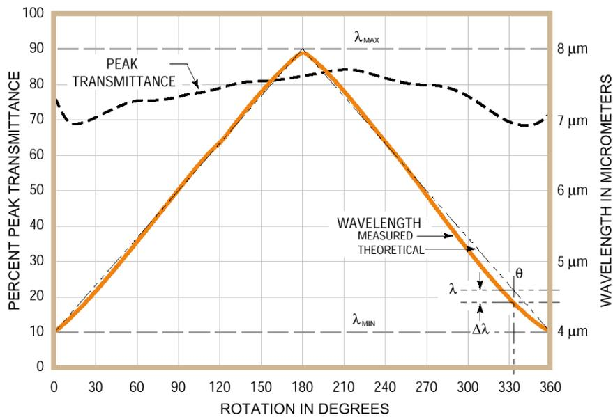
Figure 4: Typical wavelength of maximum transmittance and peak transmittance of a CVF at different angles of rotation of two 180° segments glued together (from OCLI's technical material).
