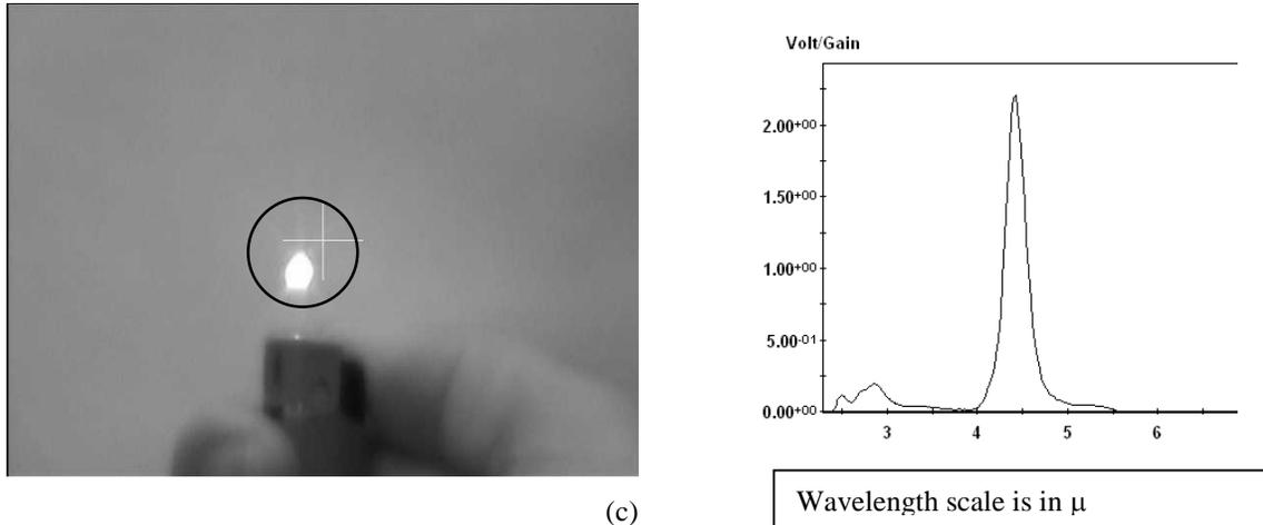
Figure 7: Three instants during the burning of a cigarette lighter, and their corresponding spectra, showing the intensity variations of the strong CO<sub>2</sub> emission line at 4.3 μ.
