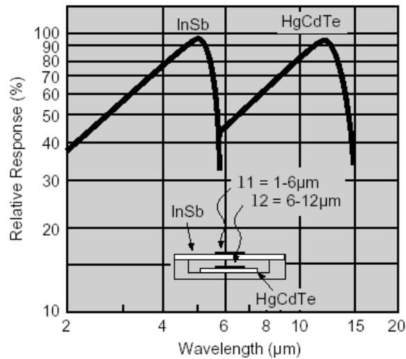
Figure 6: Typical response curve of a sandwich InSb/HgCdTe detector for maximum performance in the 2 to 15  $\mu$  region.
