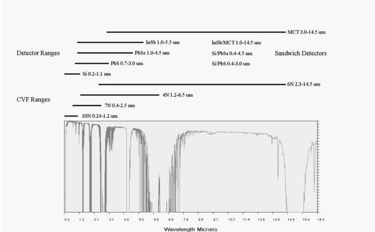
Figure 5: Atmospheric windows, and detector and CVF ranges for best spectral coverage of IR spectroradiometric measurements.
