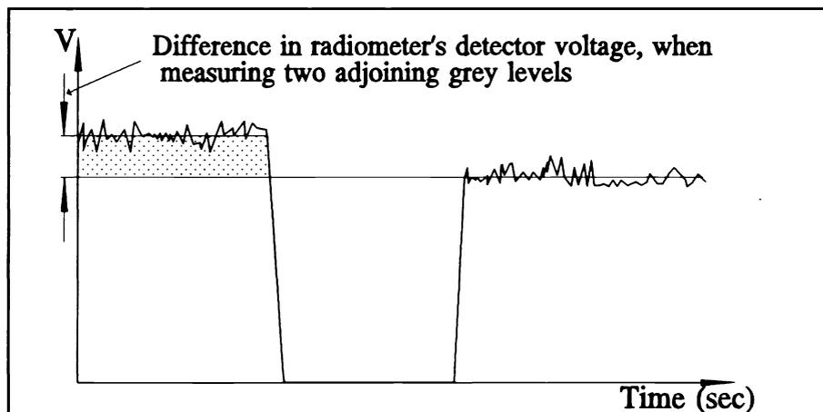
*Figure 4: Radiometric measurement of two successive grey levels.*
