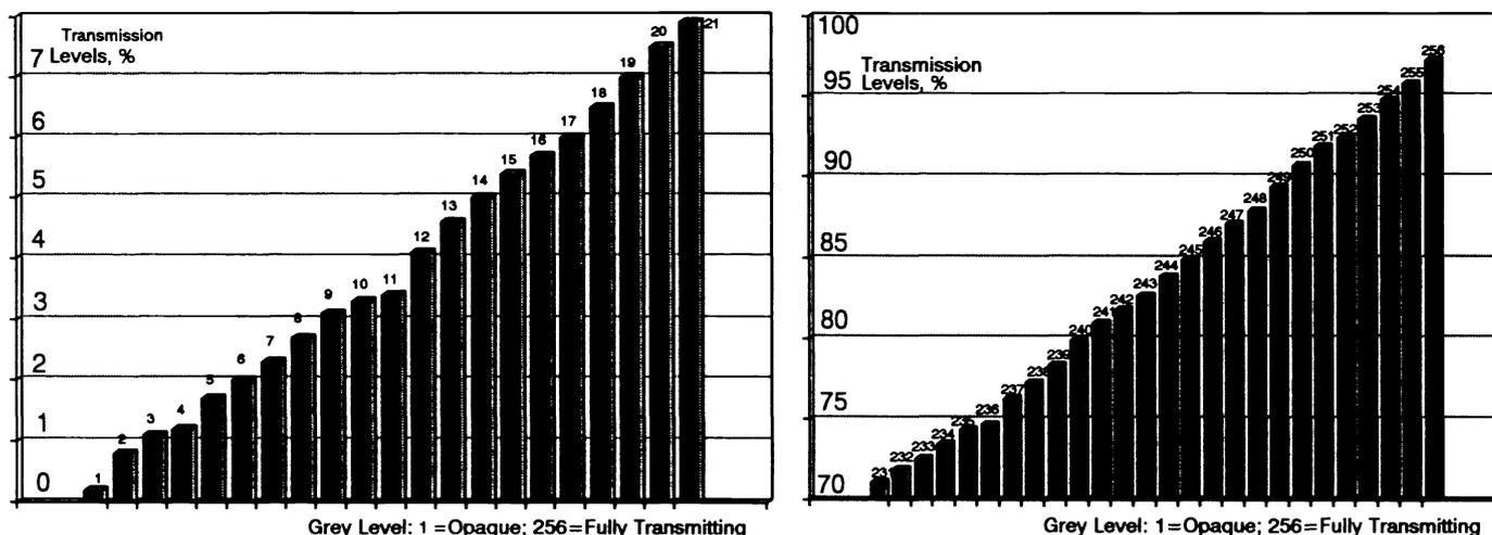
Figure 5: Levels of transmittance at the two grey level extremes. Note the higher gradient in the region (right), resulting from the doubling of the increment between the grey levels.
